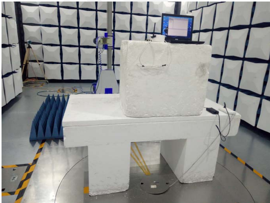
Radiated Spurious Emissions Test View (Above 1GHz)
